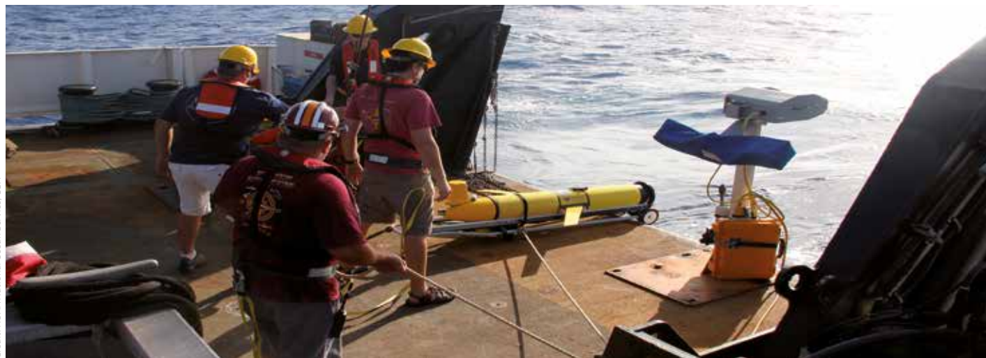
Scientists and crewmembers prepare to launch an ocean glider from the rear of the NOAA ship Nancy Foster. Once released, the pre-programmed glider will operate autonomously.
